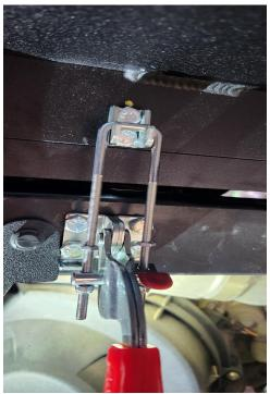
16. With the latch now installed, rout the wiring harness along the bed and connect to the tail lights on the flatbed.
