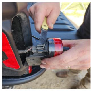
3. Remove the wiring harness from the bed until you reach the bed pivot bracket. Note: keep all tree zip tie holders on the harness, they will be used later for routing wire harness.
