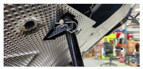
5. Now remove the four 13mm nuts holding the bed to the pivot bracket.
