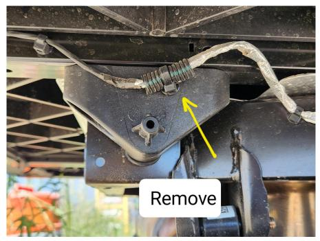
4. Once the harness is removed from the bed, tilt the bed back and remove the gas shock.
